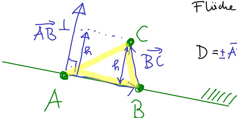
$$D = \pm \vec{AB}^\perp \cdot \vec{BC} = \pm \overline{AB} \times h$$
